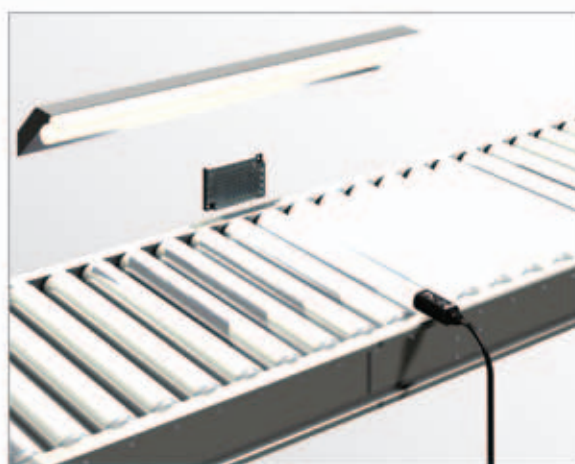
Pulse synchronisation for high ambient light immunity.
