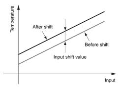
The value set for the temperature input shift is applied to the entire measurement range of the temperature sensor.
