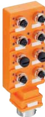
Pluggable actuator/sensor distribution box with LED operation and function indicators, 8 ports, combined FIXCON/M12 socket, 5 poles, 2 signals per socket, earth connection, central male connector with bayonet locking – especially designed for welding applications –
