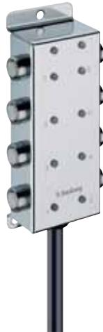
Actuator/sensor distribution box with LED operation and function indicators, housing and receptacle shells in stainless steel, with lateral ports, 8 ports, M12 socket, 4 poles, 1 signal per socket, integrated control cable – especially designed for use in food processing equipment –
