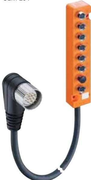
Miniature sensor distribution box with LED operation and function indicators, 8 ports, screw-lock M8 socket, 3 poles, 1 signal per socket, earth connection, integrated control cable with M23 male right angle connector, 12 poles – suitable to connect at e2c 67 I/O modules 0942 UEM 027, 0942 UEM 014 and 0942 UEM 204 –
