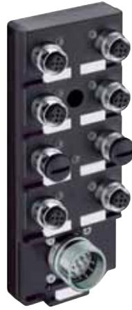
Pluggable actuator/sensor distribution box with LED operation and function indicators, to connect 4 standard sensors and 4 standard actuators with separate power supply for inputs and outputs, 8 ports, combined FIXCON/M12 socket, 4 poles, 1 signal per socket, M23 connection for the control cable
