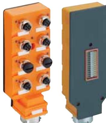
Pluggable actuator/sensor distribution box with LED operation and function indicators and terminal block with clamp terminals on the rear, 8 ports, combined FIXCON/M12 socket, 4 poles, 1 signal per socket, earth connection, central male connector with bayonet locking – especially designed for welding applications –
