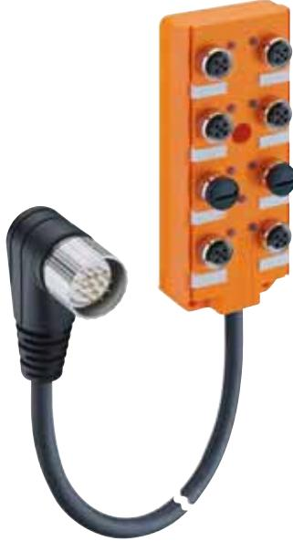
Actuator/sensor distribution box with LED operation and function indicators, 8 ports, combined FIXCON/M12 socket, 4 poles, 1 signal per socket, earth connection, integrated control cable with M23 male right angle connector, 12 poles – suitable to connect at e2c 67 I/O modules 0942 UEM 027, 0942 UEM 014 and 0942 UEM 204 –
